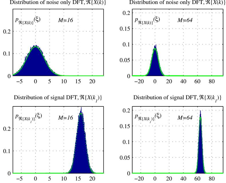
**Fig. 4:** Histograms and Gaussian probability density functions for the signal and noise only positions in the DFT for a three-component signal with  $N = 128$  and  $M = 16$  (left) and  $M = 64$  (right). The histograms are calculated in  $10^5$  random realizations of  $M$  available samples and random signal frequency positions.
