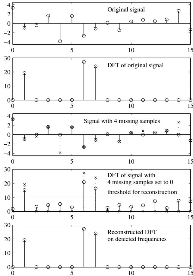
**Fig. 2:** Original signal in the discrete-time domain (first row); the DFT of the original signal (second row); signal with four missing samples at  $n = 2, 4, 11,$  and  $14$  set to zero (third row); the DFT of signal with missing values being set to 0 (fourth row). The reconstructed signal assuming that the DFT contains components only at frequencies where the initial DFT is above threshold (fifth row). Absolute values of the DFT and real part of signal are shown.
