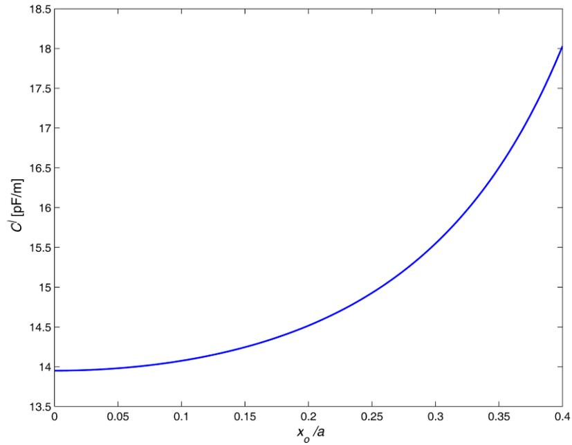
Fig. 2. Conductor capacitance versus its position.
