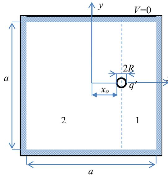
Fig.1. Thin line conductor inside grounded square shield.
