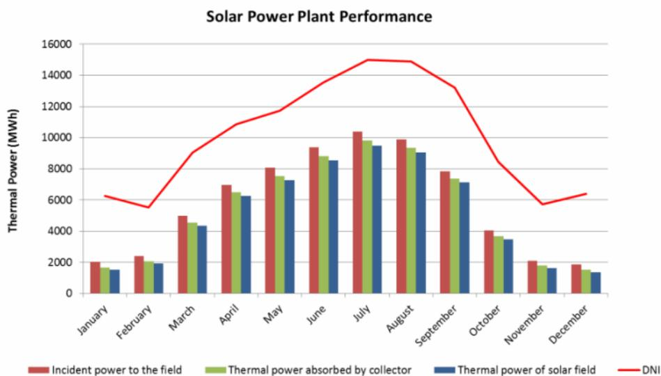
Fig. 6: Thermal performance of the solar field.
