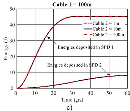
Fig. 9. Energies deposited in SPD 1 and SPD 2 for active power of 400W and different lengths of cable 1 and cable 2: a) cable 1 length of 1m, b) cable 1 length of 10m and c) cable 1 length of 100m
