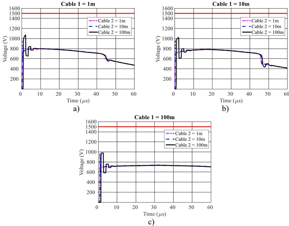
Fig. 7. Voltage across resistive load with 400W for different lengths of cables 1 and 2: a) cable 1 length of 1m, b) cable 1 length of 10m and c) cable 1 length of 100m
