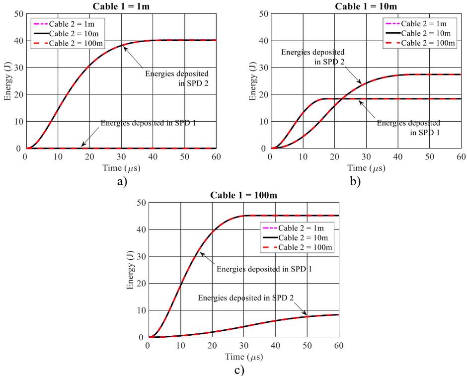
Fig. 8. Energies deposited in SPD 1 and SPD 2 for active power of 100W and different lengths of cable 1 and cable 2: a) cable 1 length of 1m, b) cable 1 length of 10m and c) cable 1 length of 100m
