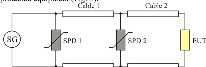
Fig. 5. Model of two-stage protection system
