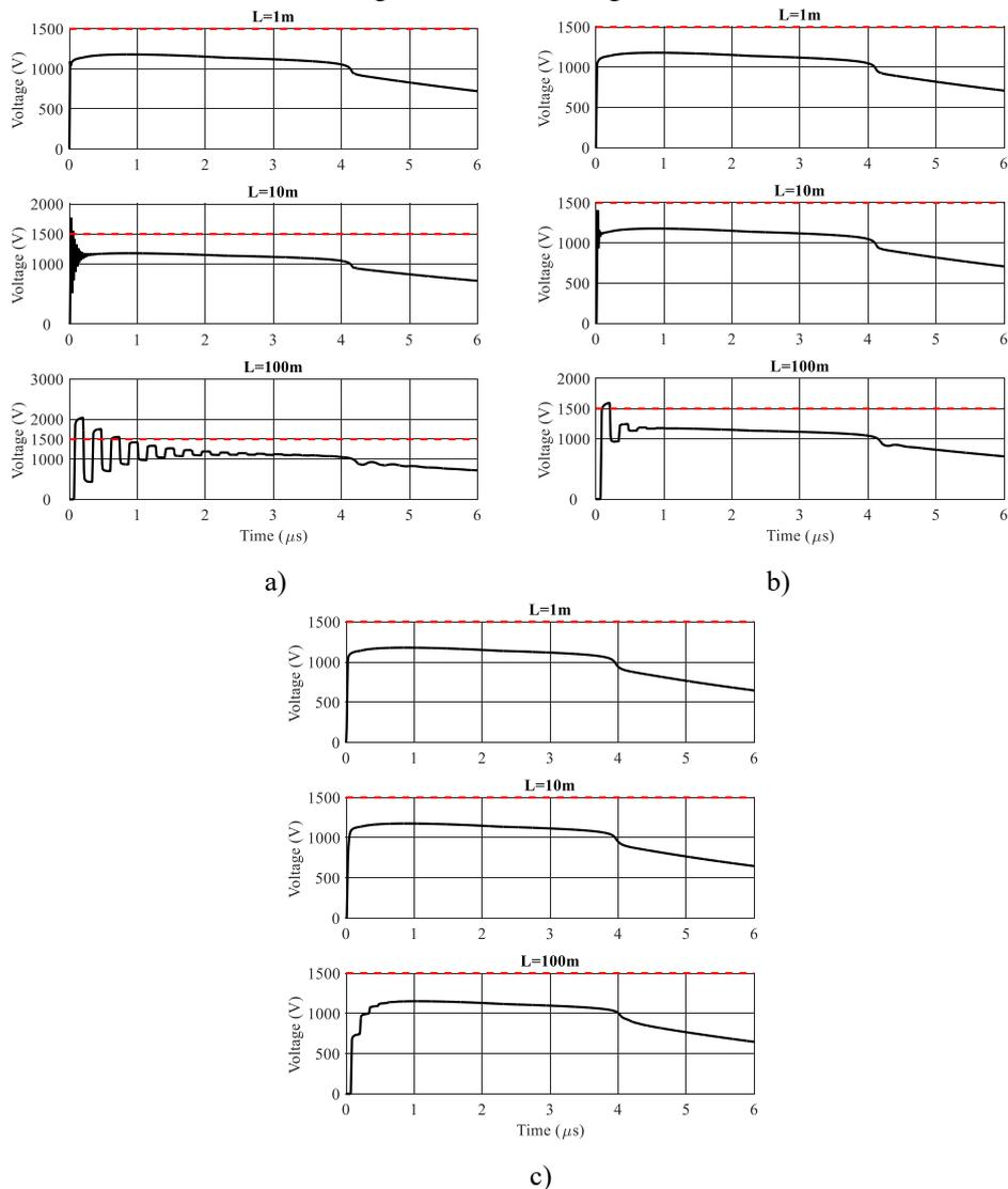
Fig. 3. Voltages across resistive load with a) 100W, b) 400W and c) 2000W for different cable lengths
