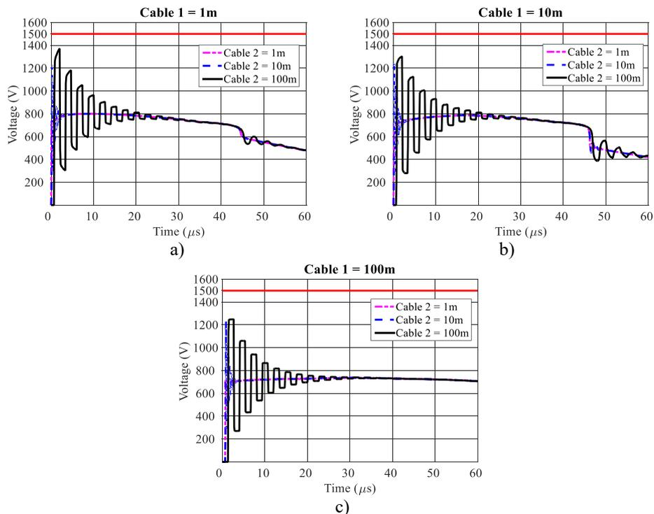
Fig. 6. Voltage across resistive load with 100W for different lengths of cables 1 and 2: a) cable 1 length of 1m, b) cable 1 length of 10m and c) cable 1 length of 100m
