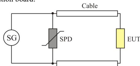
Fig. 1. Model of overvoltage protection system
