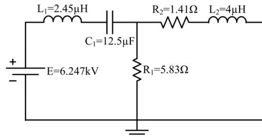
Fig. 2. Model of the Combination Wave generator
