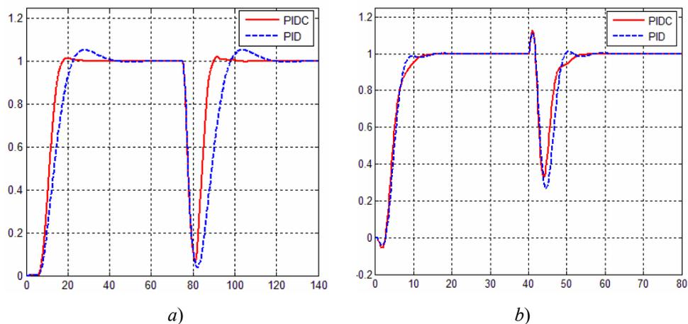
Fig. 4. Comparison of step responses to a reference signal  $r(t)=1$  and disturbance  $d(t)$  with PIDC controller (red thick line) and PID controller (blue dashed line); a)  $d(t)=1$  ( $t > 70$  s) for process  $G_{p3}(s)$  and  $b=0$ ; b)  $d(t)=1$  ( $t > 40$  s) for process  $G_{p4}(s)$  and  $b=0$
