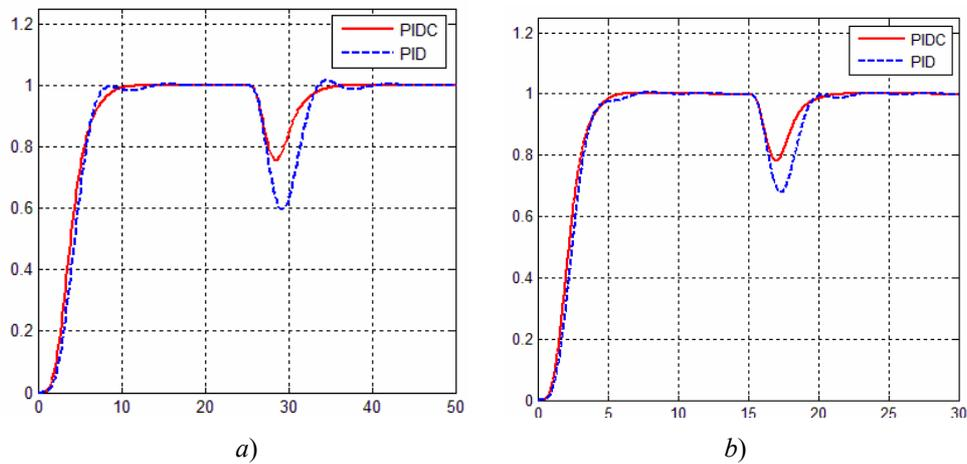
Fig. 3. Comparison of step responses to a reference signal  $r(t)=1$  and disturbance  $d(t)$  with PIDC controller (red thick line) and PID controller (blue dashed line); a)  $d(t)=1$  ( $t > 25$  s) for process  $G_{p1}(s)$  and  $b=0$ ; b)  $d(t)=1$  ( $t > 15$  s) for process  $G_{p2}(s)$  and  $b=0$
