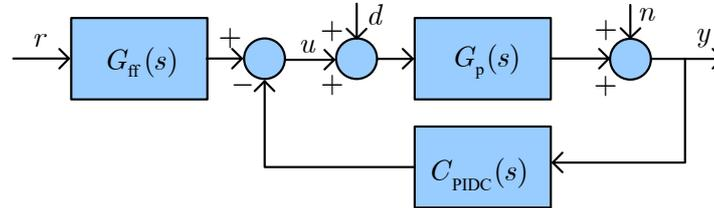
Fig. 2. Control structure with controller  $C_{PIDC}(s)$
