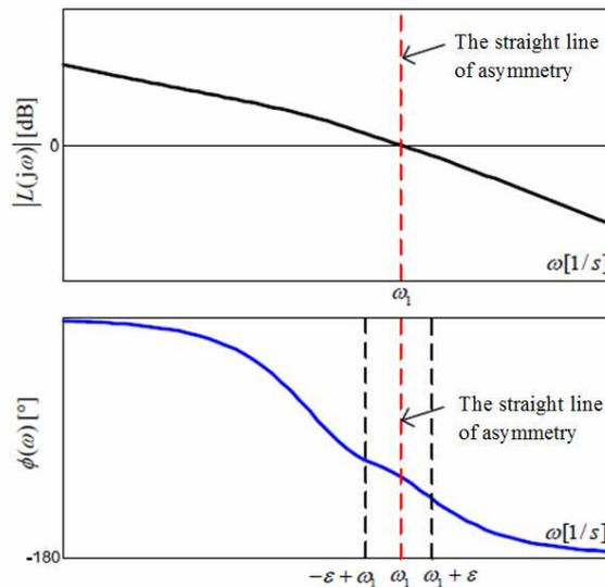
Fig. 1. Bode plots of feedback function  $L(j\omega)$  illustrating NSO principle
