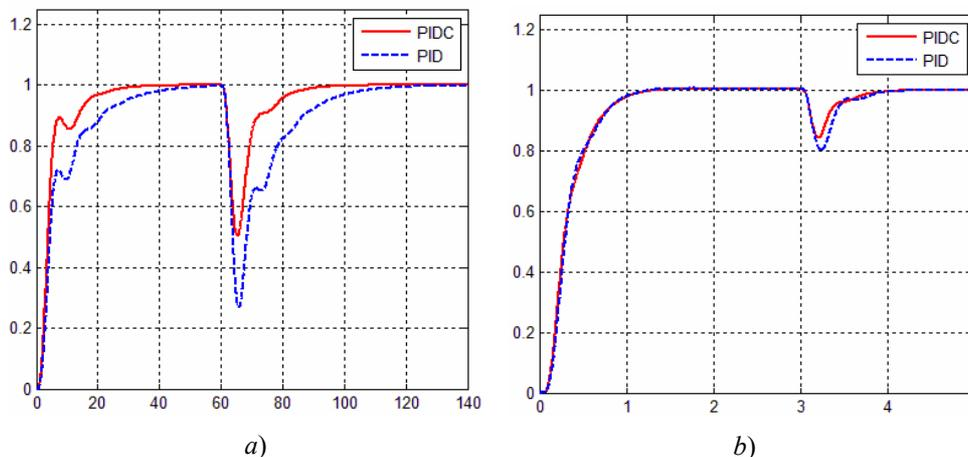
Fig. 6. Comparison of step responses to a reference signal  $r(t)=1$  and disturbance  $d(t)$  with PIDC controller (red thick line) and PID controller (blue dashed line); a)  $d(t)=0.5$  ( $\tau > 60$  s) for process  $G_{p7}(s)$  and  $b=0.4$ ; b)  $d(t)=2$  ( $\tau > 3$  s) for process  $G_{p8}(s)$  and  $b=0$
