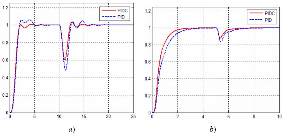
Fig. 5. Comparison of step responses to a reference signal  $r(t)=1$  and disturbance  $d(t)$  with PIDC controller (red thick line) and PID controller (blue dashed line); a)  $d(t)=1$  ( $t > 10$  s) for process  $G_{p5}(s)$  and  $b=0$ ; b)  $d(t)=1$  ( $t > 5$  s) for process  $G_{p6}(s)$  and  $b=0$
