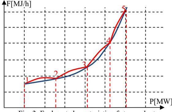
Fig. 3. Fuel cost characteristic of steam plant
