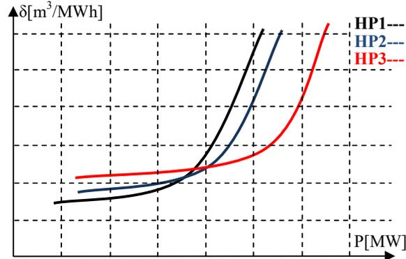
Fig. 1. Incremental water rate versus output power
