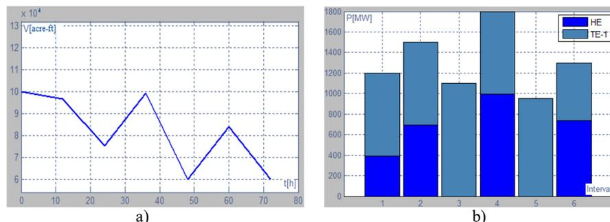
Fig.6. Results of hydro-thermal coordination: a) Deviation of accumulation volume amount, b) Optimized load distribution of power plants
